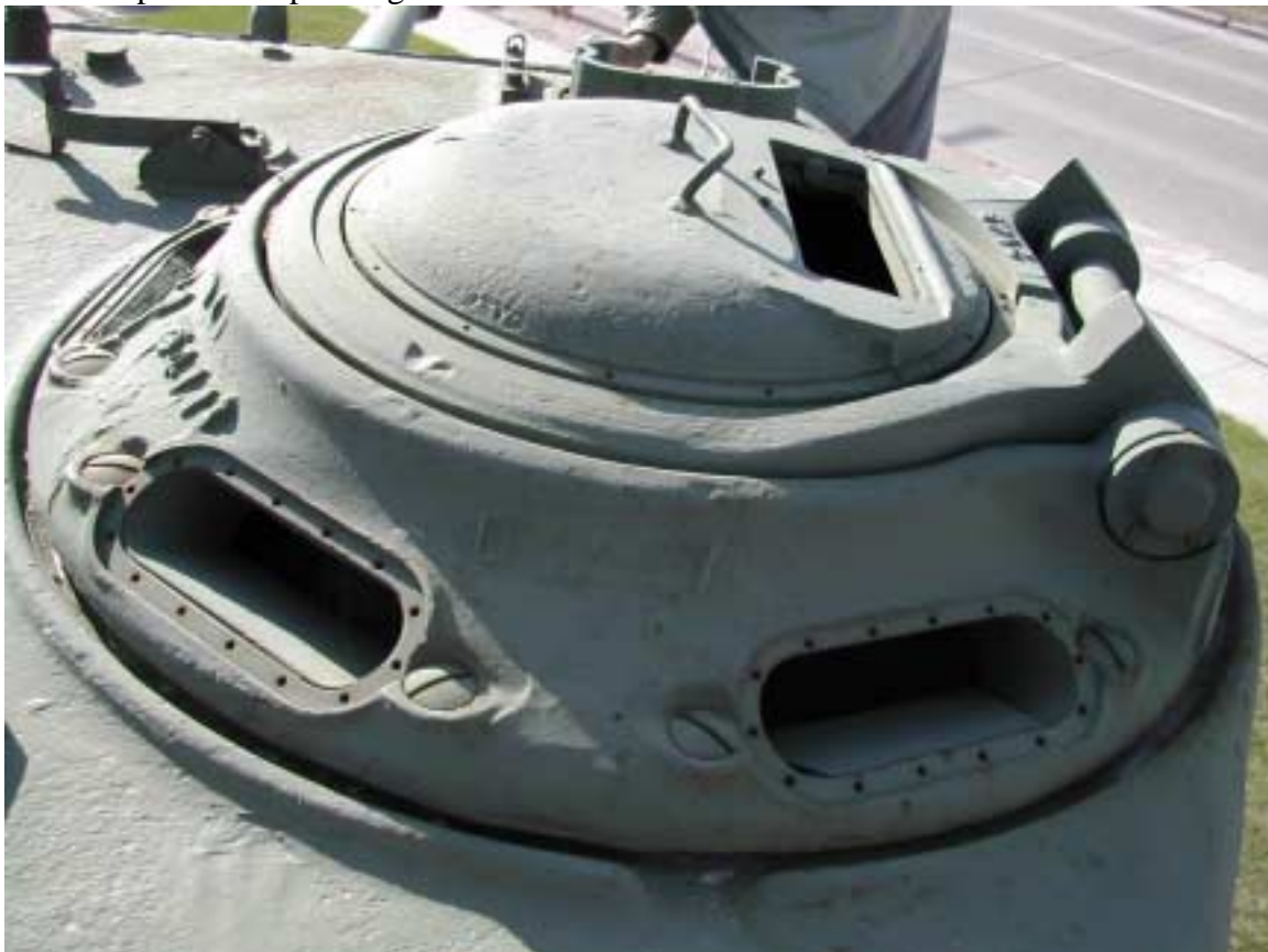
The crew-commander's cupola. Covers were made for the missing periscopes and vision blocks
