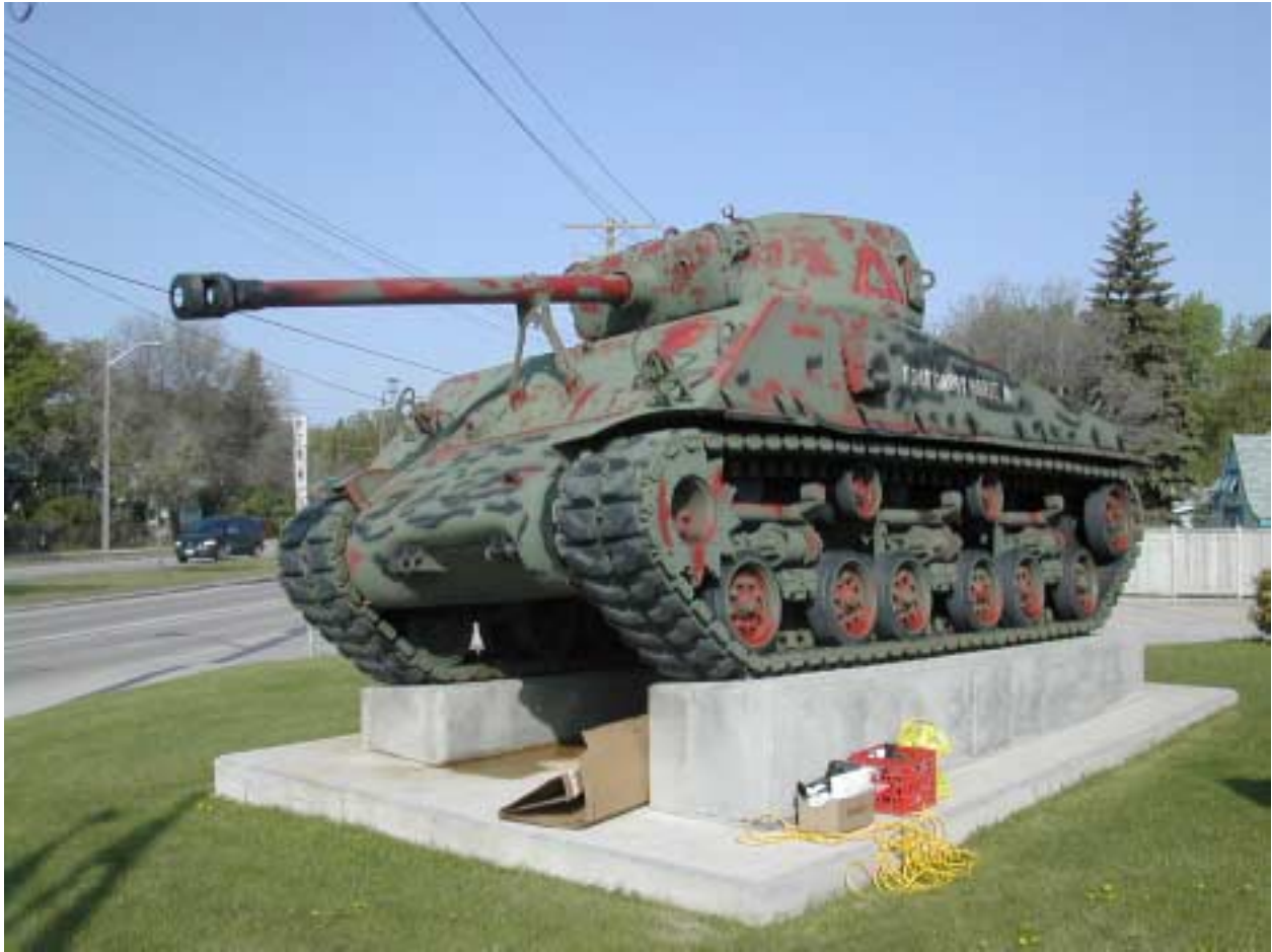
The tank with rust paint applied, prior to painting with 24087
