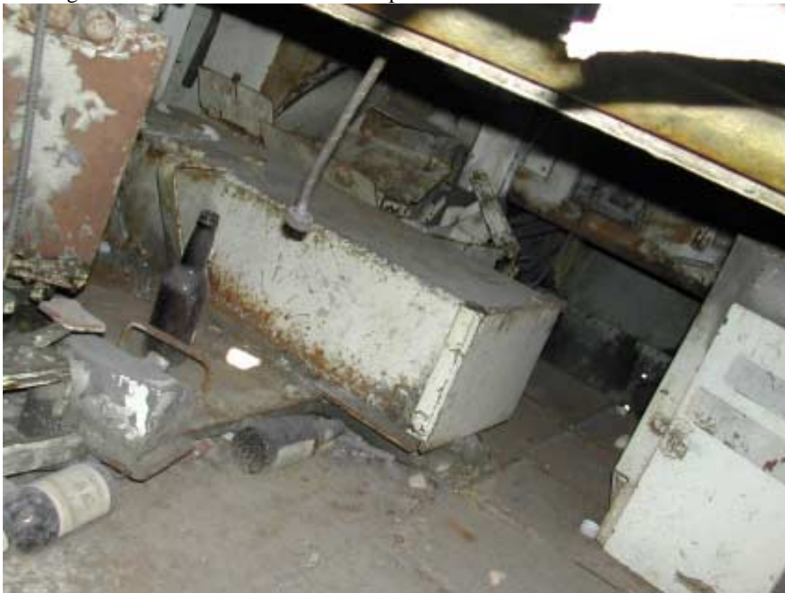
Turret floor, showing 6-round armoured ammunition bin
