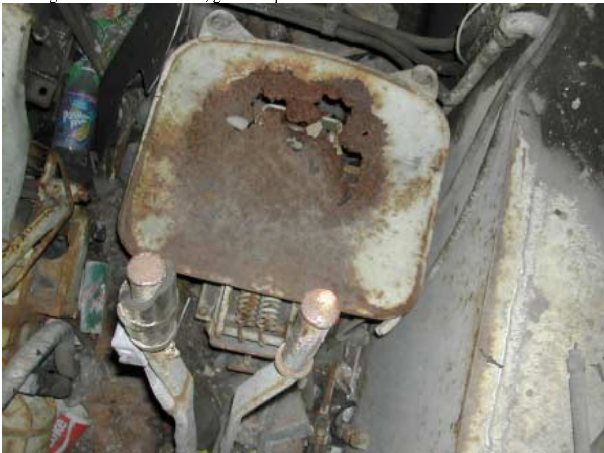
Driver's seat and tiller bars for steering
